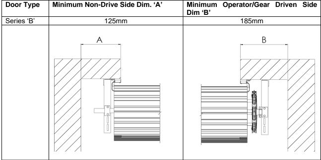
**NB:** If the door is to be motorised, check with the motor installation instructions for side room required for the motor.
