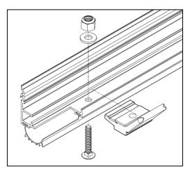
12. Secure the guide at the top allowing approximately 2-3mm running clearance per side from the edge of curtain.
