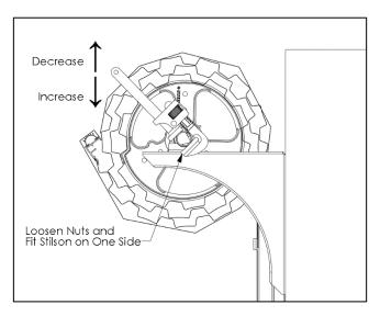
8. Carefully try the door again. It may be necessary to repeat steps 3-6 several times until the tension is correct.
