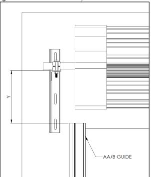
2. Fix the nylon lead-in to the top of the guide with the provided 8G-18x1<sup>1</sup>/<sub>2</sub>" self-tapping screw.
