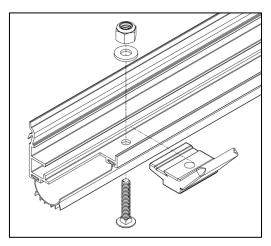
12. Secure the guide at the top slot allowing approximately 2-3mm running clearance per side from the edge of curtain.
